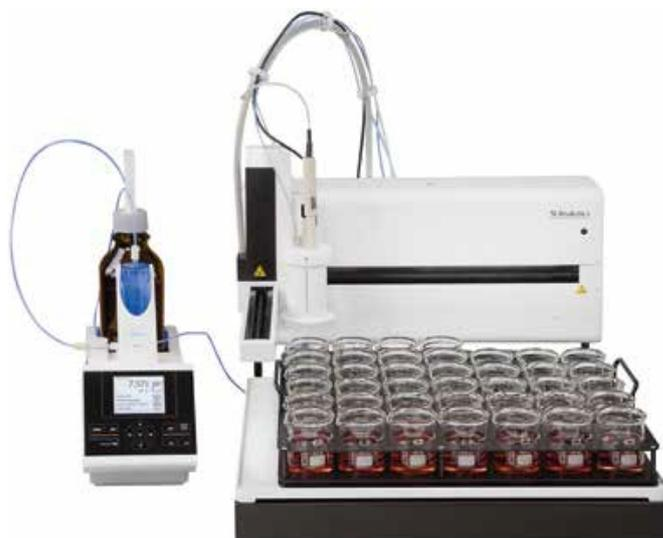
Titramax VT with connected autosampler for 42 samples
