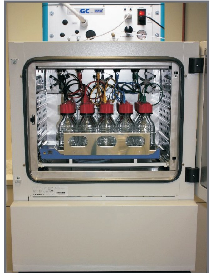
GärOnA - Incubator unit and gas chromatograph on the top
