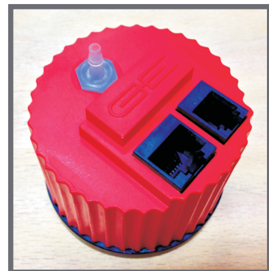
Measuring cap with integrated sensor unit
