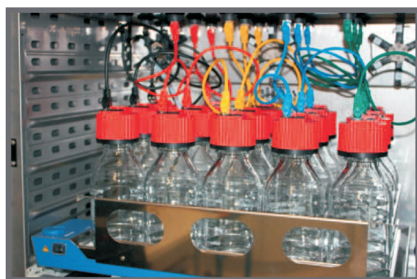
Reaction vessels with pressure transducer caps on roll-off magnetic stirrer
