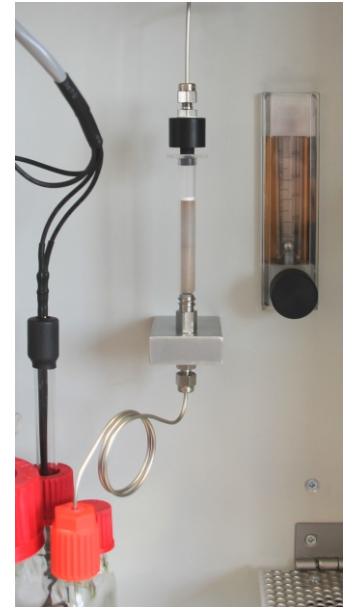
Sulphur trap for elimination of H 2 S and mercaptans
